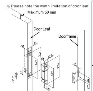
The correct installation position of the electric lock on the door leaf, not on the door frame.
