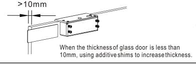
Maximum distance as 6mm. It is unable to lock if the spacing is exceeding 6mm.
