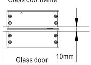
The spacing gap is suitable for 10~14mm
