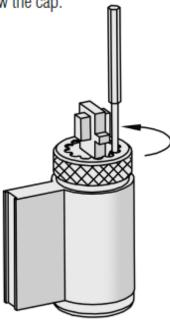
Replace the tailpiece, hold down the control pin and screw the cap fully on without tightening. Ensure control pin projects to lock the cap.
