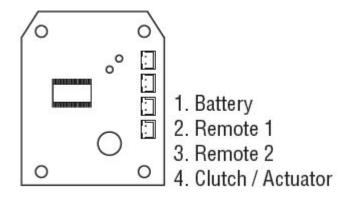
**REM 1** is intended for use when there is a need to allow a visitor to open the door after having been identified by intercom or by sight from within. **REM 1** would be connected to a pushbutton on a reception desk, or to the appropriate button on an intercom. Pushing the button would cause the Blue LED to light and would release the lock for the normal set time.
